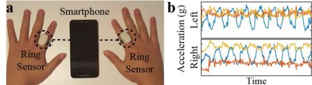
Figure 1. a) The proposed system. Each ring sensor sends data to the smartphone via Bluetooth Low Energy. b) An acceleration time series (open and closed fist) streamed from the sensor to the phone.
